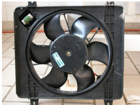
(a) Modified radiator fan
